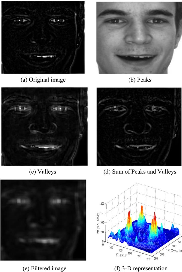
**Fig. 2** Result of eye image after morphological filtering **a** Original image **b** Peaks **c** Valleys **d** Sum of peaks and valleys **e** Filtered image **f** 3-D representation
