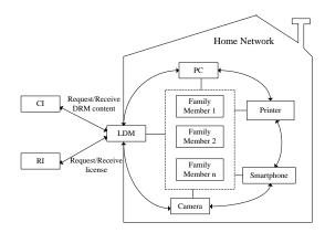
Figure 4. A DRM functional architecture for home network
