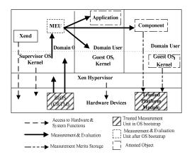
Figure 2. Xen-based Platform Architecture for AP<sup>2</sup>RA Model and Fundamental Data Streams Inclued the Platform
