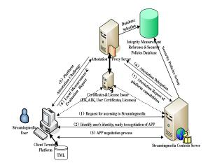
Figure 3. A framework of Trusted Distribution of Streaming Media Contents Based on Trusted Computing
